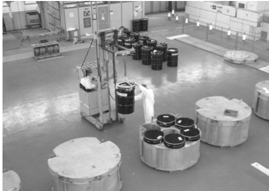
Figure 1. Standard 227 litre drum being loaded into a carousel
